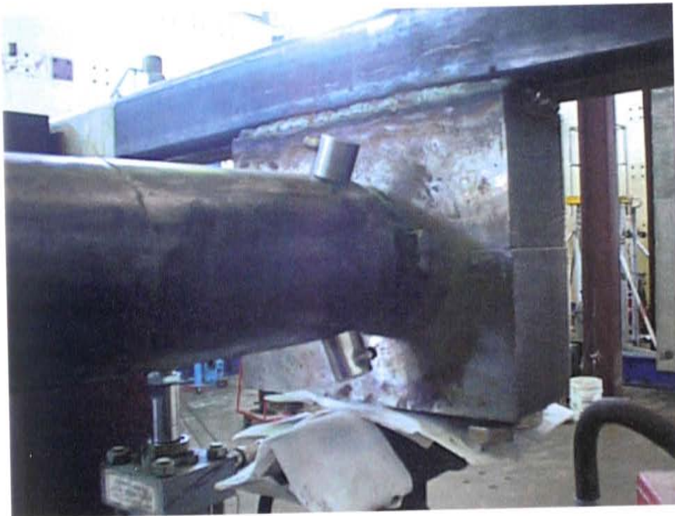
Figure 3.17: Mounted Sensors at Front of Shaft
