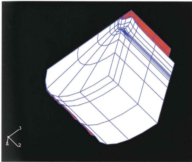
Figure 4.4: Crack at the end of 95 in-kip Fatigue Load Level
