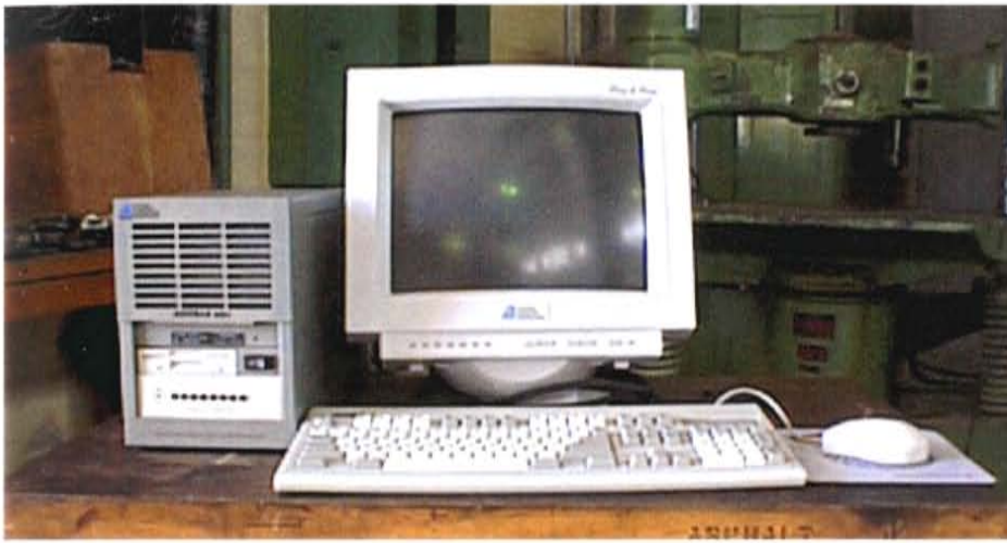
Figure 3.7: MISTRAS-2001 Digital Acoustic Emission Instrument
