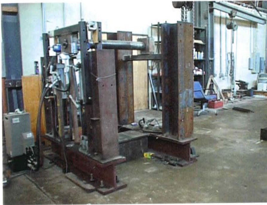
Figure 3.10: Test Frame Modified for Dynamic Loading
