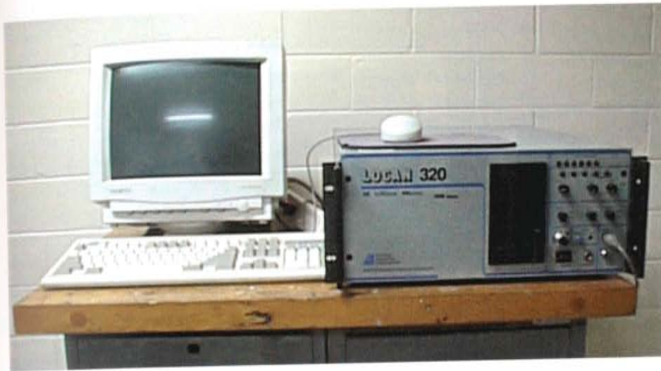
Figure 3.6: LOCAN AT Analog Acoustic Emission Instrument
